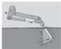
Verti-Drain's patented parallelogram design shatters the soil. Coring tines are also available on all models.
